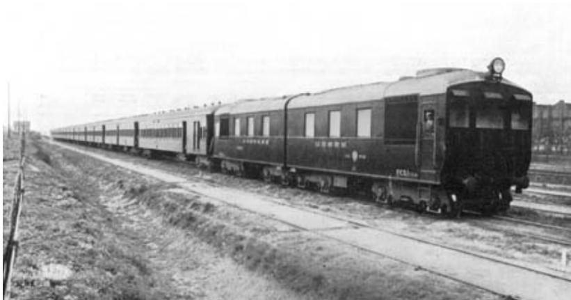
*A view from a 1933 issue of Diesel Railway Traction advertising Sulzer diesel engines shows the two 1,700hp mobile power houses with a lengthy train.*
