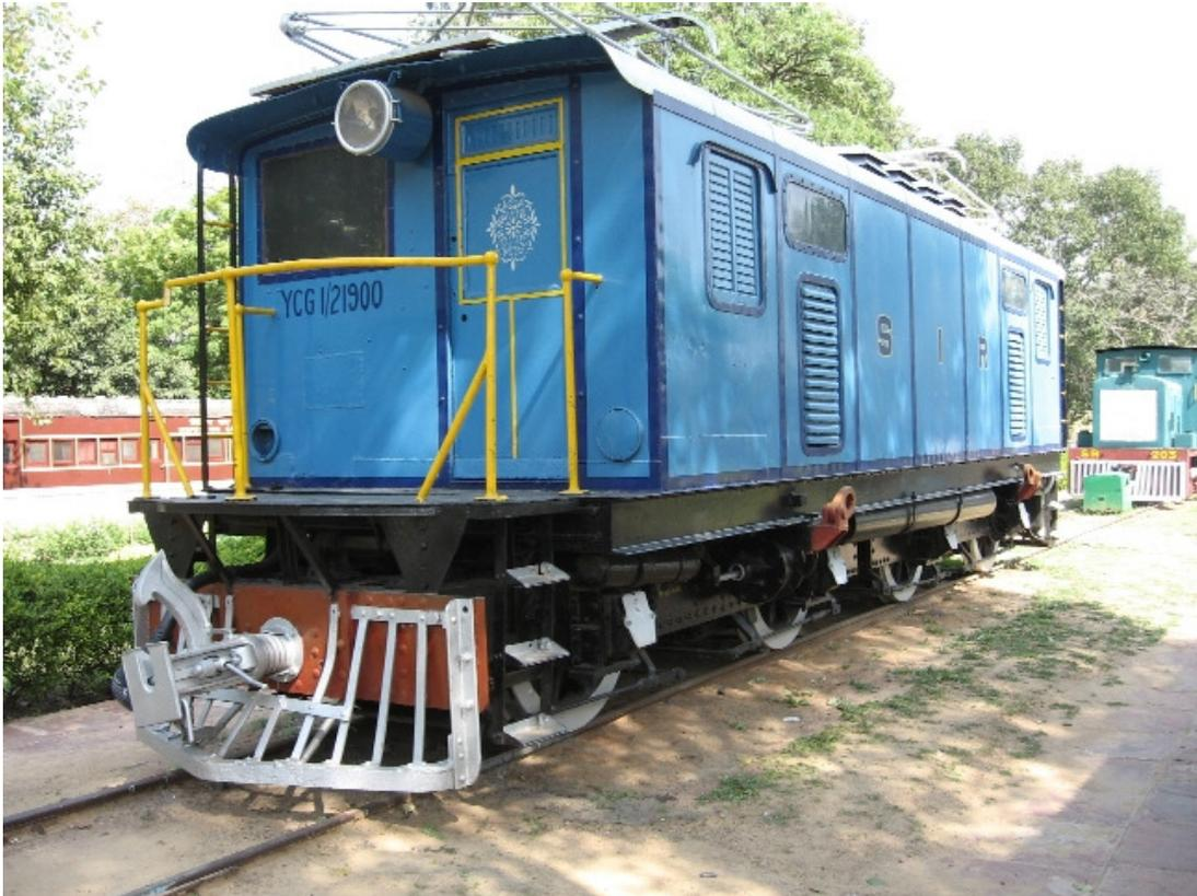
Builder: Hawthorn Leslie & Co, UK. Electricals by English Electric, Leeds, UK Class: YCG/1 Year Built: 1930 Service: SIR (South Indian Railway), later SR (Southern Railway) Wheel Arrangement: Bo-Bo Unique Features: Dual braking (vacuum and air), entrance from balconies at each end.
