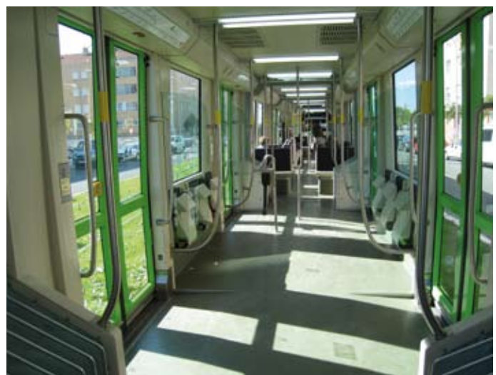
Below right: The interior layout on the 100% low floor provides ample space for wheelchairs and pushchairs, with fold down seats.
