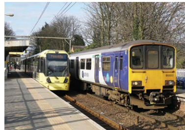
▲ ABOVE: Navigation Road's separate tracks for Metrolink and national rail. The latter hosts freight and infrequent Manchester - Chester passenger services; a similar single Metrolink platform operation exists at Newton Heath and Moston stop.
