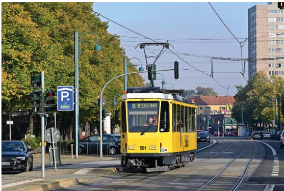
▲ Not in public service... former Berlin T6A2M501, a rail grinder nicknamed 'Schleiff', runs along Karl-Marx-Strasse in October 2020. Robert Bartkowiak
