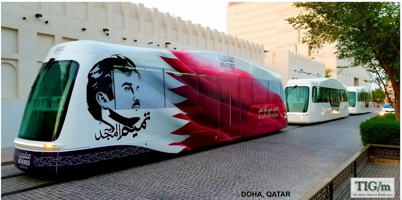
MRV-3 City Car single car body and is rated to carry 100 pax and can be coupled autonomously as above to a maximum of three as shown above and using suitable, safe sidings and unneeded car 2 or 3 can be parked off peaked eliminating unnecessary dead mileage and wear and tear.
