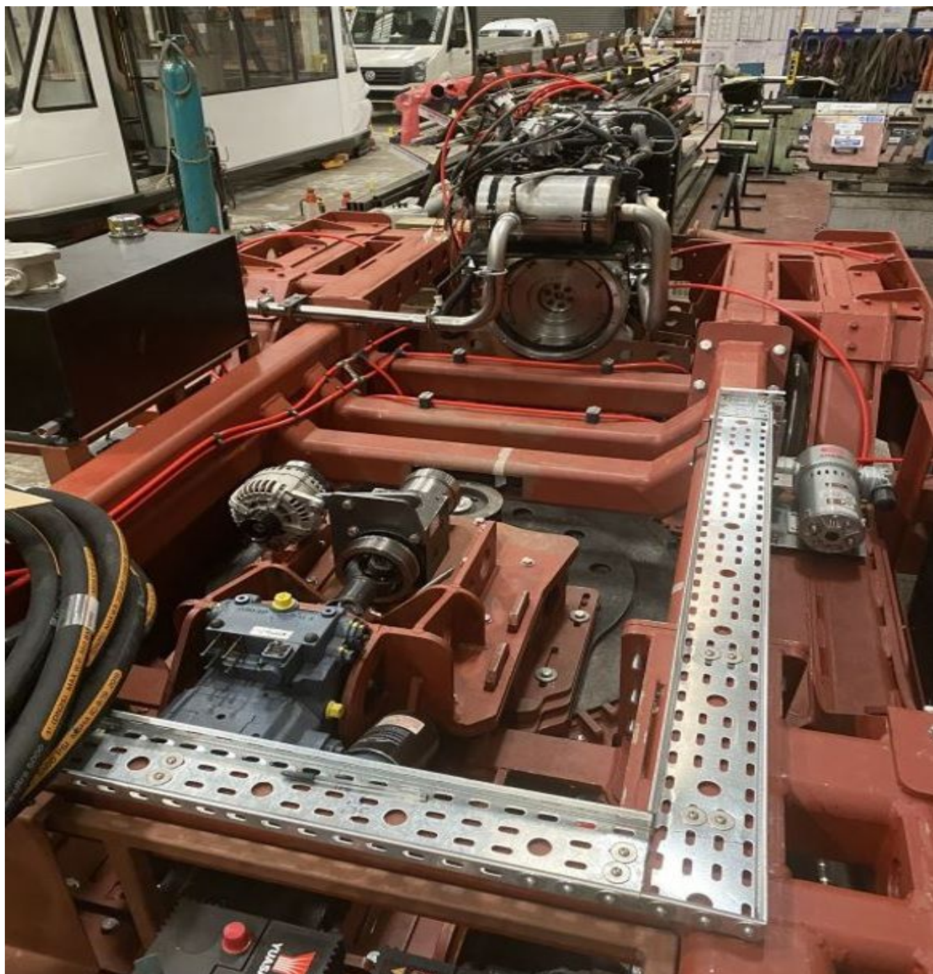
Pictured: Engine mounted and integrated into bogie; Primary & Secondary driveline integrated into bogie
