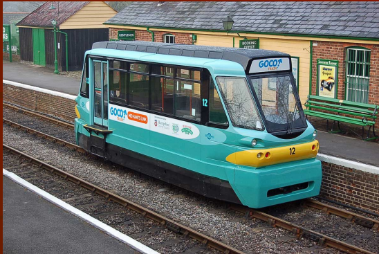
Taunton Car 139012 (Tram version available) Diesel & Flywheel Into service Stourbridge 2023
