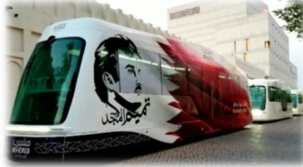
Doha VLR in Service x 100 Pax can be autonomously coupled x 3 cars
