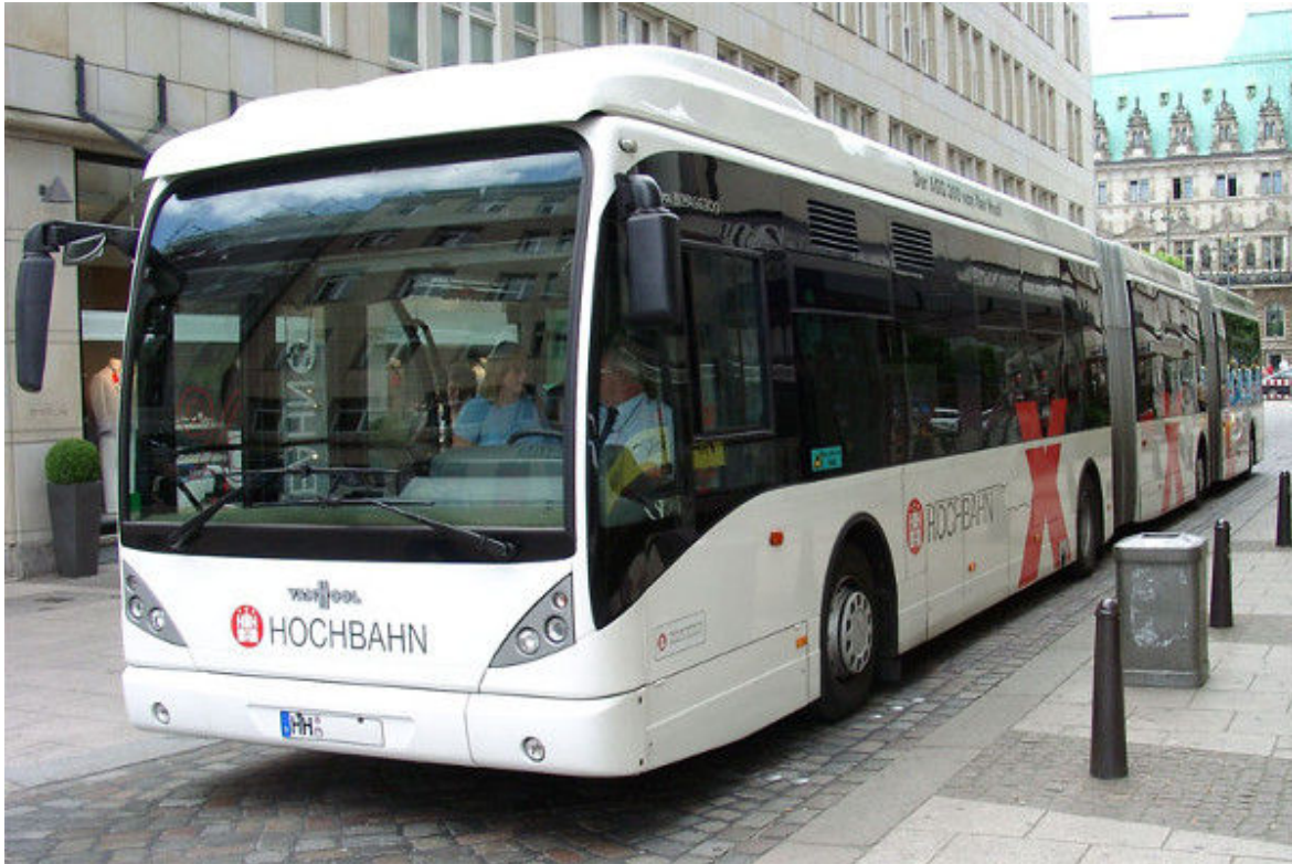
Bi-articulated Bus design by Van Hool with a length of 25 metres (Image Credit: Van Hool)
