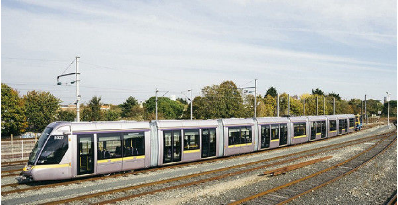
Alstom's Citadis Model 403 LRV for the streets of Dublin with a length of 55 metres (Image Credit: International Railway Journal)
