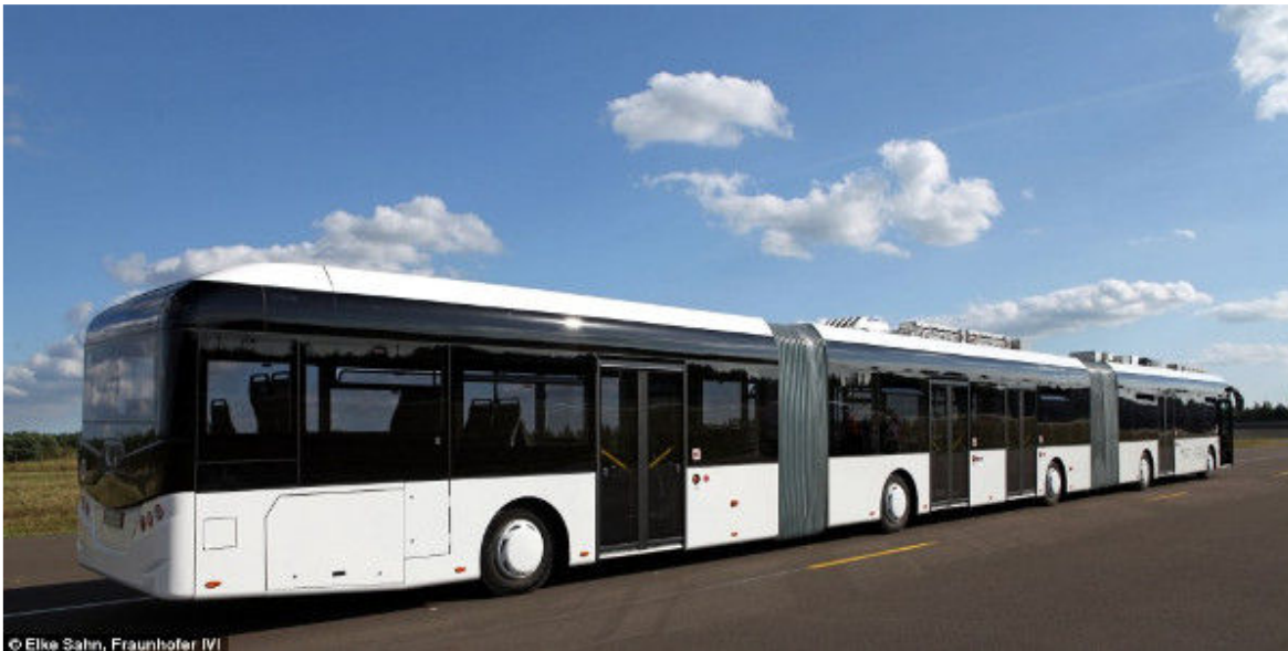
Hess of Switzerland and their Little Tram Bi-articulated Bus Series Prototype, with a length of 30 metres (Image Credit: Hess of Switzerland)
