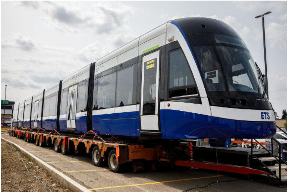
Bombardier's larger 7 section Flexity Swift Light Rail Vehicle for Edmonton with a length of 42 metres
