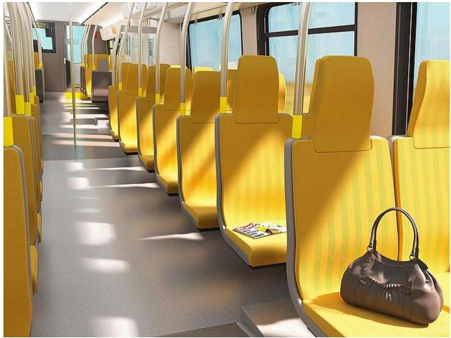
There will be a mix of airline and facing seats, with more space for bicycles, pushchairs and persons with reduced mobility. The train body will be designed specifically for the Merseyrail network, with lower floors and a sliding step to provide near-level access.
