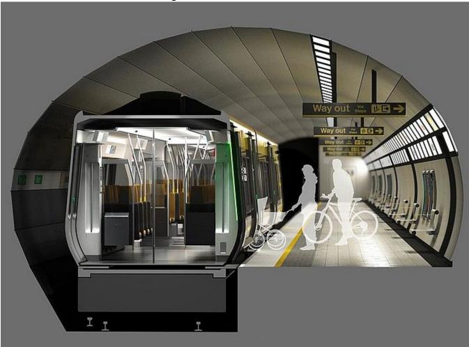
At 99 tonnes, the EMUs will be lighter than the current 105 tonne trains, and energy consumption is expected to be 20% lower, including regenerative braking; options for energy storage are to be studied.
