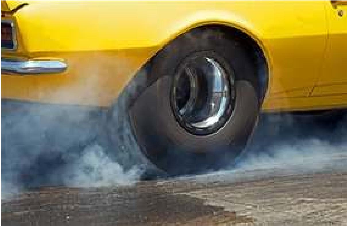
Black mark: Each time a tyre rotates, it loses a layer of rubber about a billionth of a metre thick. (Source: rcyoung/iStockphoto)
